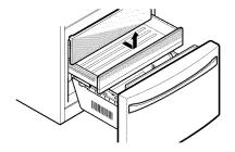
2. To replace, slightly tilt up the front of the drawer, insert the drawer into the frame, and push it back into place.
